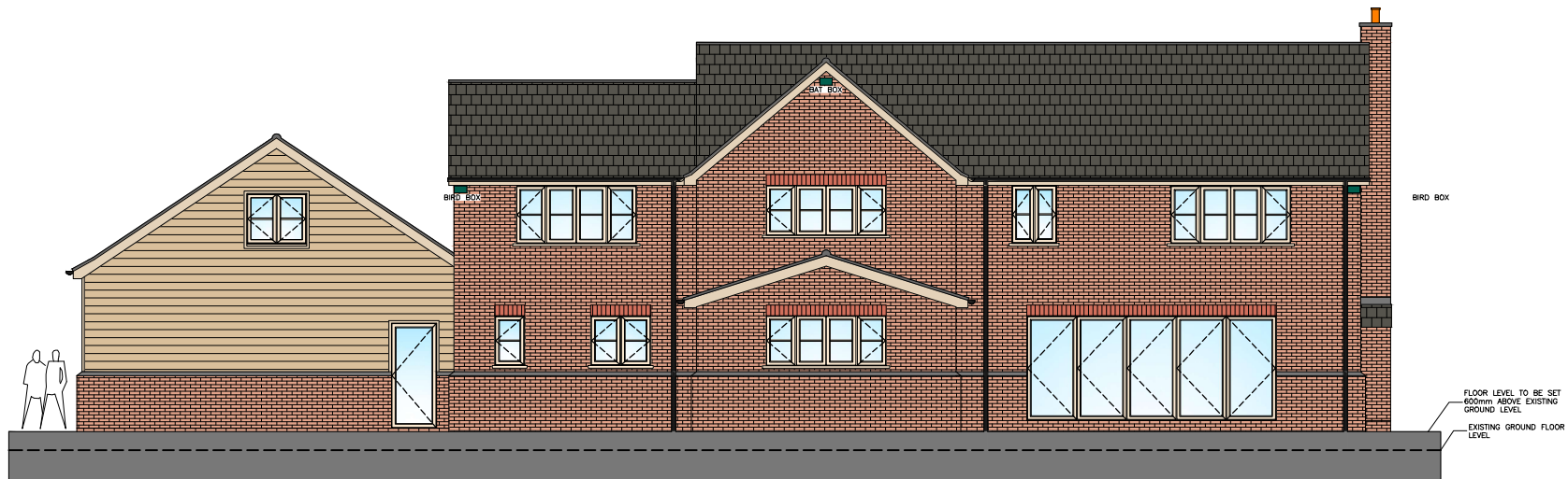
PROPOSED REAR ELEVATION (1:50)
